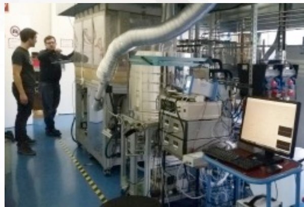
Fig. 3. ENEA gasification and EPFL/SP stack SOFC test rig
